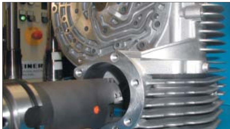
Fig 4 PCD boring bar as a combination tool with adjustable indexable inserts (for bore diameters of 76.2 mm and 82 mm)
