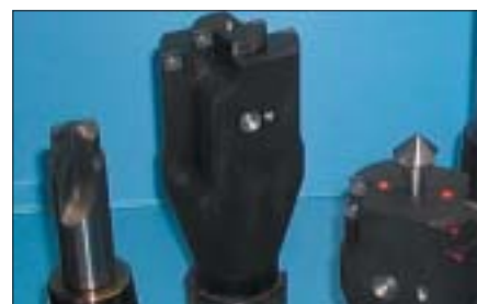
Fig 5 PCD tools are used for both roughing and finishing
