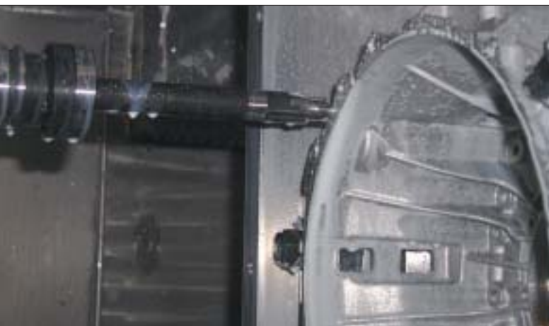
Fig 3 Machining the bore in the first set-up
