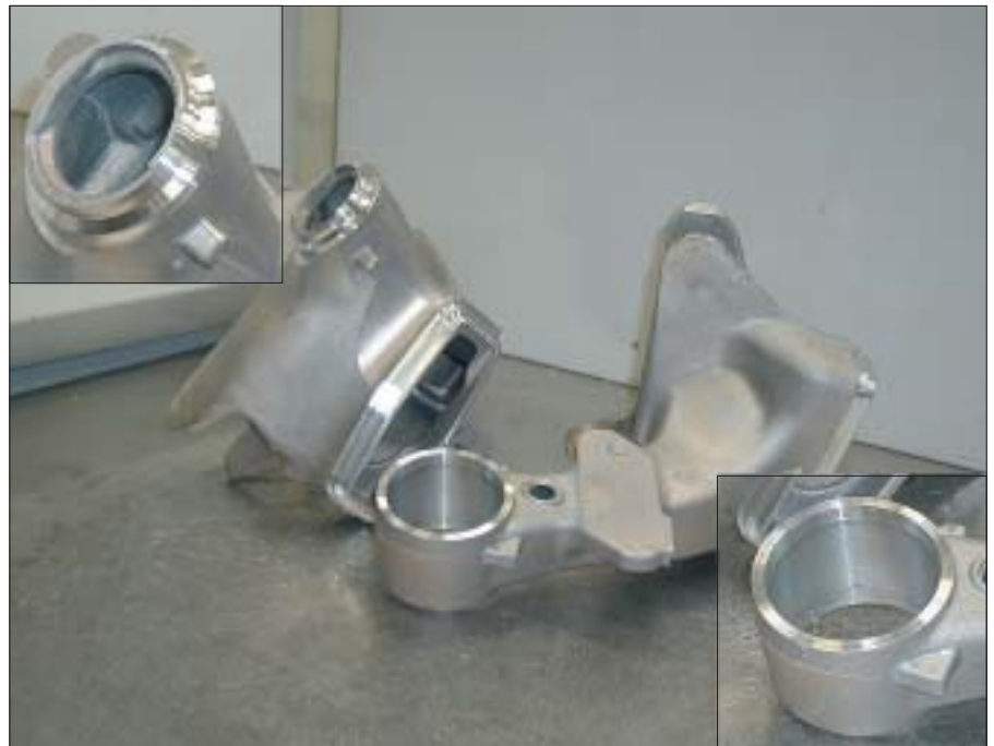
Fig 3 Faces to be machined on the right and left aluminium cast joints
